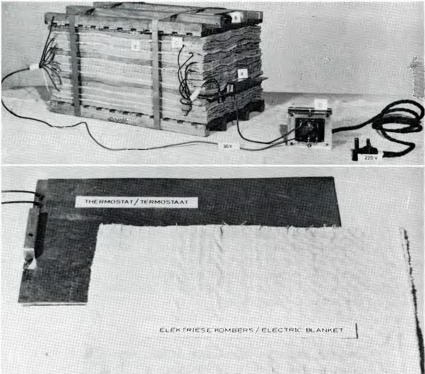
Fig. 25. **Upper**, Electric drying press for drying herbarium specimens: **A**, thermostat, **B**, indicator light, **C**, electric blanket, **D**, transformer (primary 220 V/ secondary 30 V) and **E**, drying paper. **Lower**, electric blanket and thermostat.
