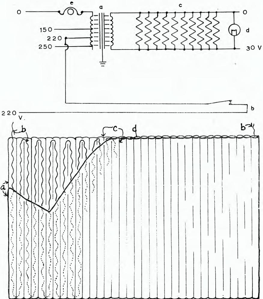
Fig. 26. Electric drying press for herbarium specimens: **Upper**, diagram of wiring of electric press: **a**, transformer; **b**, thermostat; **c**, 220 V/600 W resistance (10); **d**, indicator light; and **e**, fuse.
